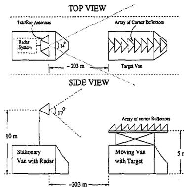
Figure 2: Geometry of field experiments for Doppler measurements.
