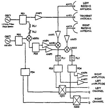
Figure 1: Block diagram of coherent ultrawideband random noise radar.
