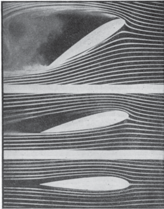
Fig. 9-9 Smoke is used in the NACA smoke tunnel at Langley Field, Virginia, to make the flow of air visible, as illustrated in these photographs. Note the smoothness of the air flow in the lowest picture. When the angle of attack has been increased to 10^\circ , the air flow begins to separate from the upper surface of the airfoil (center view); and when the angle is increased to 30^\circ , the flow separates completely from the upper surface. Turbulence behind the trailing edge of the airfoil may be observed in this picture. (Reproduced from the Journal of Applied Physics , August, 1943, with permission of the National Advisory Committee for Aeronautics.)
