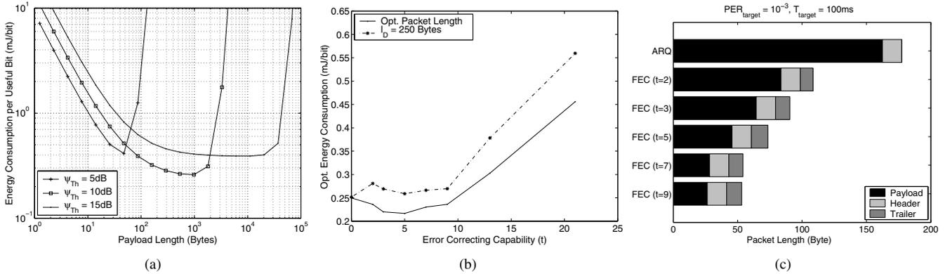
Fig. 2. Energy per useful bit (6) vs. payload length for (a) ARQ and (b) Energy consumption per bit with optimum packet length and  $l_D = 250$  bytes., and (c) optimal packet length for different error control techniques.
