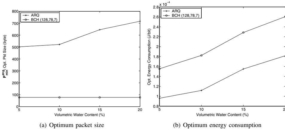
Fig. 5. Optimization results for  $P_{min}^{eng}$  in underground environment as a function of volumetric water content.
