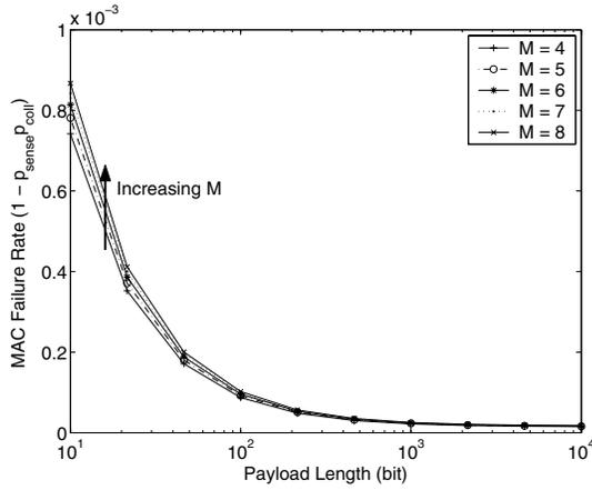
Fig. 1. MAC failure rate vs. payload length for different values of  $M$ .
