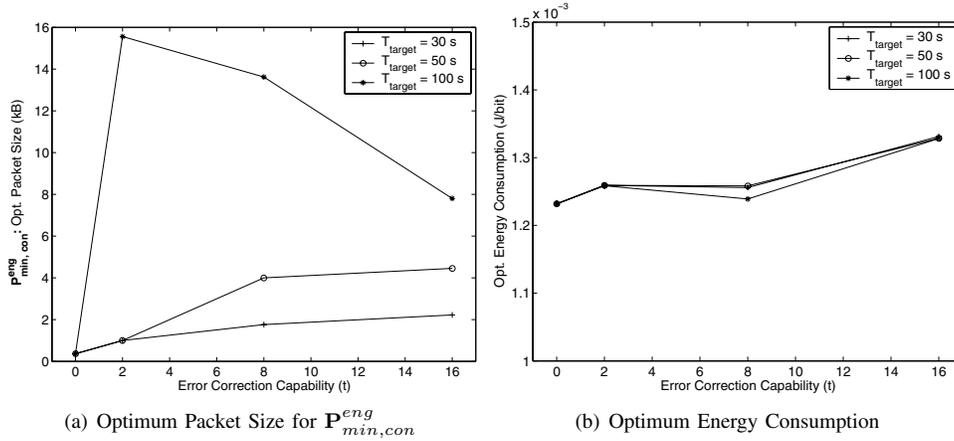
Fig. 4. Constrained optimization results as a function of error correction capability,  $t$ , for different delay bounds in shallow water.
