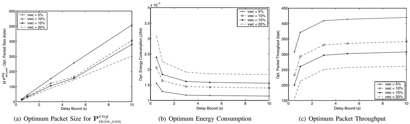
Fig. 6. Constrained optimization results as a function of end-to-end delay bound in underground environment for volumetric water content.
