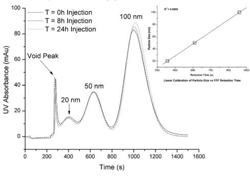
**Fig. 1.** Overlay of triplicate FFF-UV fractograms of polystyrene bead calibration standards. FFF separation conditions were 1.0 mL/min channel flow and 0.75 mL/min cross flow. UV absorbance detection is at 254 nm wavelength. Inset: Linear regression calibration function using 20, 50, and 100 nm polystyrene bead standards. Error bars represent standard deviation of the triplicate retention times obtained from UV absorbance data at maximum absorbance.
