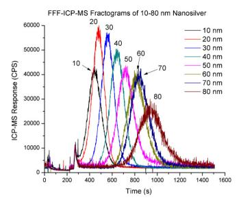
**Fig. 3.** Individual FFF–ICP-MS fractograms overlain of NanoXact silver nanoparticles. Each peak represents  $200 \,\mu\text{g/L}$  total silver as nanosilver particles. FFF separation conditions were  $1.0 \,\text{mL/min}$  channel flow and  $0.75 \,\text{mL/min}$  cross flow with ICP-MS detection using  $^{107}$  Ag.
