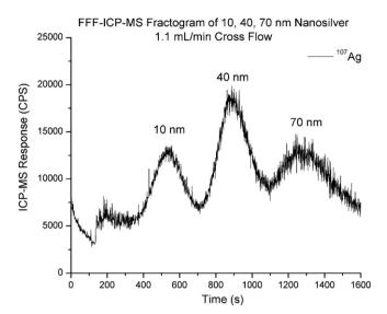
**Fig. 5.** FFF–ICP-MS fractogram of a mixture of 10, 40, and 70 nm silver particles at  $67 \,\mu\text{g/L}$  each. FFF separation conditions were  $1.0 \,\text{mL/min}$  channel flow and  $1.1 \,\text{mL/min}$  cross flow with ICP-MS detection using  $^{107}\text{Ag}$ .
