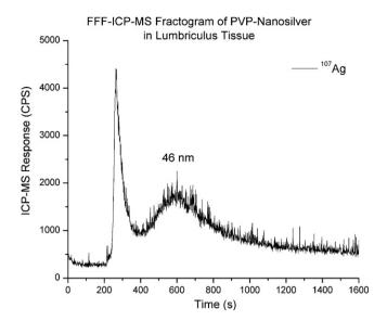
**Fig. 7.** FFF–ICP-MS fractogram of a PVP-coated silver nanoparticle extracted from *Lumbriculus* tissue by sonication in deionized water. FFF separation conditions were  $1.0 \, \text{mL/min}$  channel flow and  $0.75 \, \text{mL/min}$  cross flow with ICP-MS detection using  $^{107} \text{Ag}$ .
