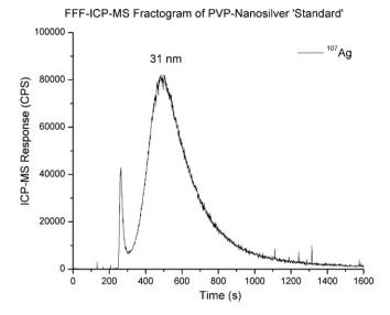
**Fig. 6.** FFF-ICP-MS fractogram of the stock PVP-coated silver nanoparticle in deionized water. FFF separation conditions were 1.0 mL/min channel flow and 0.75 mL/min cross flow with ICP-MS detection using <sup>107</sup>Ag.
