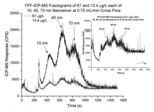
**Fig. 4.** FFF-ICP-MS fractograms of a mixture of 10, 40, and 70 nm silver particles at 67 and  $13.4\,\mu g/L$  each. FFF separation conditions were  $1.0\,m L/m$ in channel flow and  $0.75\,m L/m$ in cross flow with ICP-MS detection using  $^{107}$ Ag. Inset: FFF-ICP-MS fractogram of a mixture of 10, 40, and 70 nm silver particles at  $6.7\,\mu g/L$  each. FFF separation conditions were  $1.0\,m L/m$ in channel flow and  $0.75\,m L/m$ in cross flow with ICP-MS detection using  $^{107}$ Ag.
