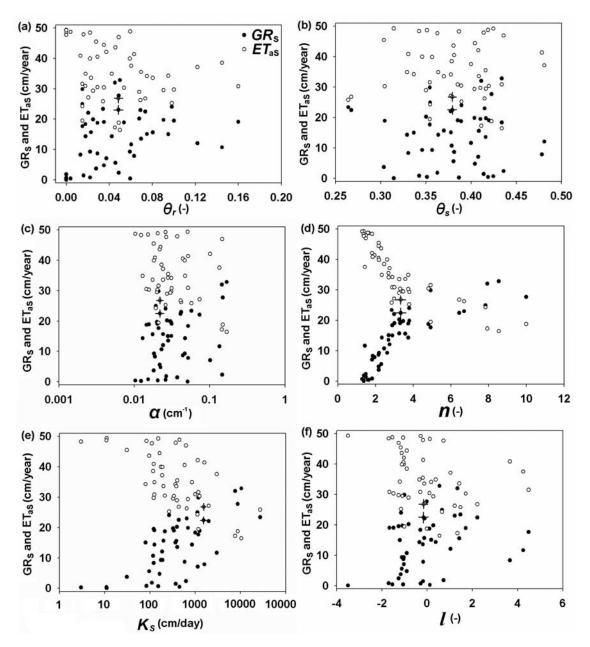
**Figure 5.** Sensitivity analysis of groundwater recharge (GR<sub>S</sub>) and actual evapotranspiration ( $ET_{aS}$ ) of sand to the van Genuchten parameters: (a)  $\theta_r$ , (b)  $\theta_s$ , (c)  $\alpha$ , (d) n, (e)  $K_s$ , and (f) l. Pluses represent results from mean SHCs.
