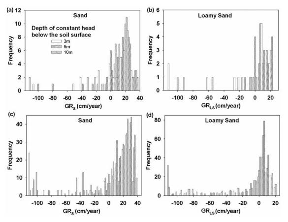
**Figure 7.** Distributions of groundwater recharge (GR) under the constant head conditions: (a) sand and (b) loamy sand from the measured data set and (c) sand and (d) loamy sand from the uncorrelated data set. Bin size is 5 cm/a.
