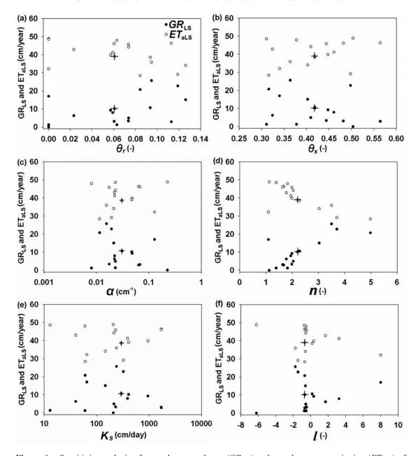
**Figure 6.** Sensitivity analysis of groundwater recharge (GR<sub>LS</sub>) and actual evapotranspiration ( $ET_{aLS}$ ) of loamy sand to the van Genuchten parameters: (a)  $\theta_r$ , (b)  $\theta_s$ , (c)  $\alpha$ , (d) n, (e)  $K_s$ , and (f) l. Pluses represent results from mean SHCs.
