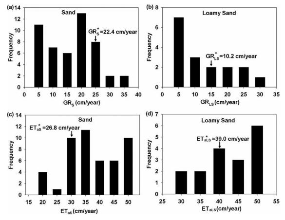
**Figure 3.** Distributions of groundwater recharge (GR) for (a) sand and (b) loamy sand and actual evapotranspiration ( $ET_a$ ) for (c) sand and (d) loamy sand based on the measured data set under the unit gradient flow boundary condition. The asterisk represents the results based on mean SHCs. Bin size is 5 cm/a.
