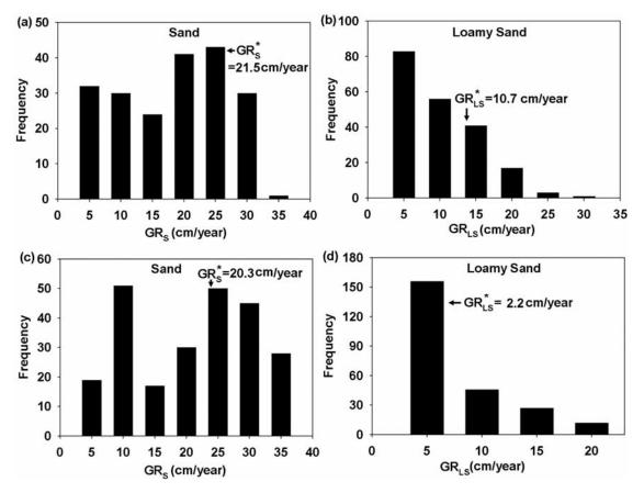
**Figure 4.** Distributions of groundwater recharge (GR) under the unit gradient flow lower boundary condition: (a) sand and (b) loamy sand from the correlated data set and (c) sand and (d) loamy sand from the uncorrelated data set. The asterisk represents the results based on mean SHCs. Bin size is 5 cm/a.
