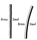
**Fig. 14-6** Bending of a bimetallic strip when heated.
