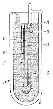
Fig. 14-3 Diagram of the National Bureau of Standards triple-point cell, BD, in use in an ice bath G, within a thermos flask H. A, water vapor; C, thermometer well; E, ice mantle; F, liquid water.
