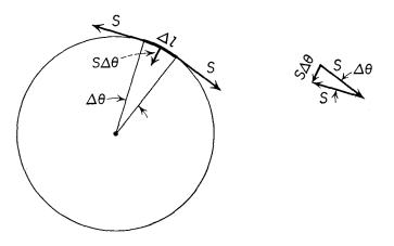
**Fig. 14-11** The radial force exerted by a circular hoop under tension S upon a section of length  $\Delta l$  is given by  $S\Delta\theta$ , where  $\Delta\theta$  is the angle subtended by the section  $\Delta l$  at the center of the circle.
