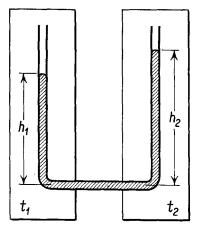
Fig. 14-9 Dulong and Petit apparatus.
