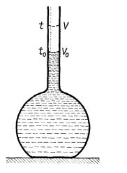
**Fig. 14-8** Expansion of a liquid in a container when heated.
