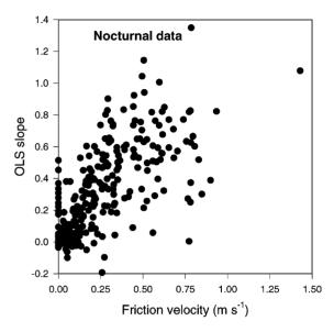
Fig. 4. The OLS slope against friction velocity  $(u_*)$  during nocturnal periods (net radiation less than zero). Each site-year is represented by five points, representing data sorted by friction velocity into five 20 percentile groups of half-hour data.
