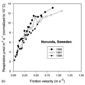
Fig. 10. The mean nocturnal respiration, normalized to  $10\,^{\circ}$ C, against friction velocity sorted into 20 five percentile friction velocity groups using the method of Falge et al. (2001): (a) data from agricultural field in Bondville, IL; (b) data from a mixed forest in Norunda, Sweden.
