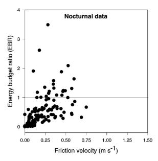
Fig. 6. EBR against friction velocity  $(u_*)$  during nocturnal periods (net radiation less than zero). Each site-year is represented by five points, representing half-hour data sorted by friction velocity into five 20 percentile groups.
