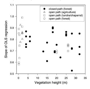
Fig. 1. The slope of the OLS regression against vegetation height for sites using closed (closed symbols) and open (open symbols) path IRGAs. Symbol shapes represent different vegetation types.
