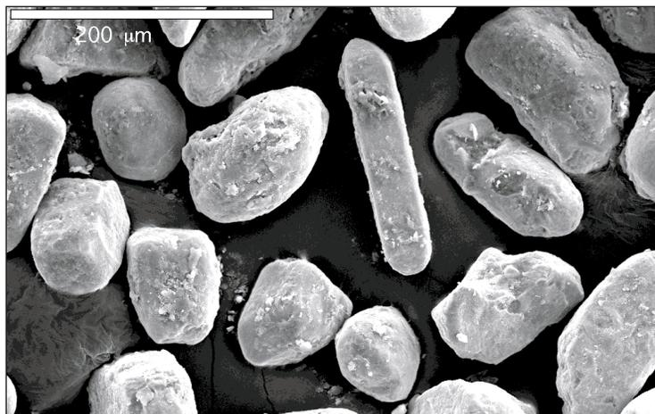
**Figure 2.** Scanning electron microscope digital image of zircon from loess sample Li-210, collected at a depth of about 5 m at the Beecher Island locality. Elongate prismatic zircon has morphology characteristic of 34 Ma volcanic zircon from the White River Group. More rounded grains are typical of the Proterozoic population found in both the loess and White River Group.
