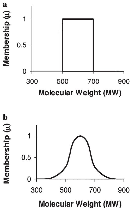
**Figure 1.** Membership functions of (a) a crisp set and (b) a fuzzy set. The crisp set includes all compounds with a molecular weight (MW) of 500 to 700 and assigns them a membership value of one. All other compounds with an MW outside that set have membership equal to 0. The fuzzy set includes the set of compounds with an MW "around 600."
