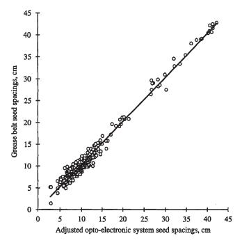
**Figure 4.** Comparison of 508 adjusted seed spacings from the opto-electronic system with spacings measured from the grease belt for all the spacings from all the test runs for the regular-pelleted and mini-pelleted sugarbeet seeds, and pelleted chicory seeds with a planter travel speed of 3.2 km/h. The regression analysis showed a coefficient of determination  $(r^2)$  of 0.977 with a slope of 0.991 and an intercept of 0.19 cm.
