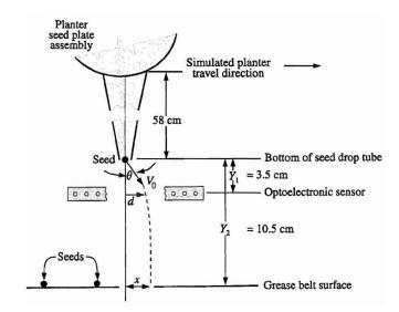
**Figure 3.** Side view schematic diagram showing the adjustment to the optoelectronic sensor spacing to improve its representation of the seed spacing at the grease belt.  $V_0$  = seed velocity;  $\theta$  = angle of deflection from vertical; d = horizontal translation of seed at sensor; x = horizontal translation of seed at belt;  $Y_1$  = fall distance from bottom of seed tube to middle of sensor;  $Y_2$  = fall distance from bottom of seed tube to belt.
