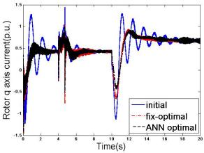
Fig.10. Simulation results of rotor q axis current I<sub>qr</sub>
