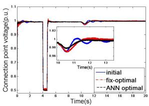
Fig.8. Simulation results of connection point voltage  $v_{\text{s}}$
