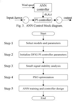
Fig. 4. Flowchart of ANN optimal DFIG model design procedure.
