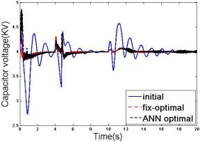
Fig. 9. Simulation results of DC-link capacitor voltage v<sub>dc</sub>
