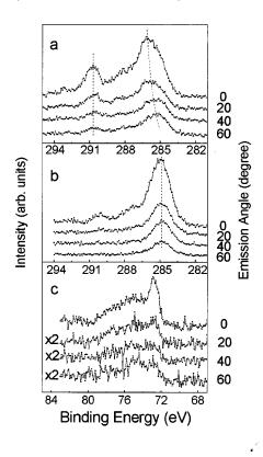
FIG. 1. Angle-resolved x-ray photoemission spectra for a 5 ML crystalline PVDF-TrFE copolymer thin film. The C 1s core level from clean PVDF-TrFE as a function of emission angle (a), the angle resolved C 1s core level at several different emission angles following aluminum deposition and 6 h annealing at 393 K (b), as well as the Al 2p core level immediately following deposition on PVDF-TrFE at room temperature (c) are shown.
