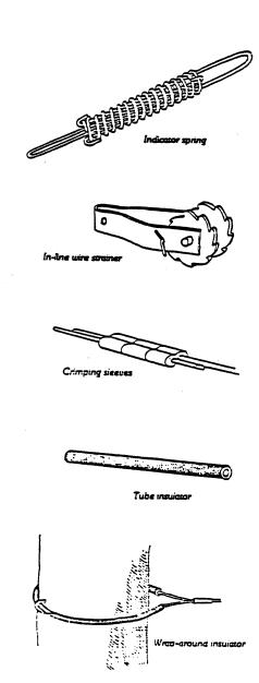
Figure 3. Components for the Penn State Vertical Electrical Deer Fence.
