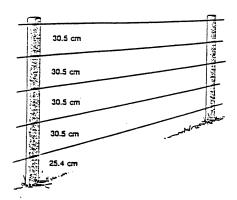
Figure 1. The Penn State Vertical Electric Deer Fence.
