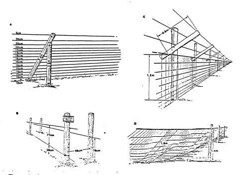
Figure 2. Other fence designs tested: A. Slanting, high-tensile, deer fence; B. Modified, New Hampshire, electric deer fence; C. Modified, stock fence; D. Slanting, or over-hanging, deer fence.
