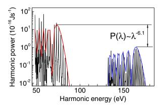
FIG. 1 (color online). HHG spectra for the H atom for  $I=2\times 10^{14}~\rm W/cm^2$  and two laser-field wavelengths,  $\lambda=1.0~\mu m$  (left) and  $\lambda=1.6~\mu m$  (right). Thin lines: numerical TDSE results; thick lines: analytic results obtained using Eq. (8).
