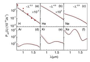
FIG. 2 (color online). Harmonic power,  $P_{\Delta E}(\lambda)$  [cf. Eq. (14)], vs  $\lambda$  for H and the rare gases with  $I=2\times 10^{14}$  W/cm² and two energy intervals  $\Delta E$ : 20 (solid lines) and 30 eV (dotted lines). Circles and squares in panel (a) mark the TDSE results for  $\Delta E=20$  and 30 eV, respectively.
