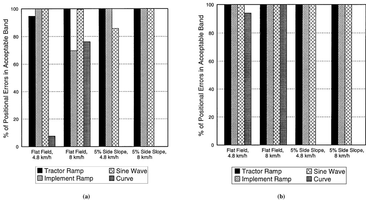
Figure 5—Percentages of tractor positional errors within (a)  $\pm 3$  cm ( $\pm 1.2$  in.), and (b)  $\pm 5$  cm ( $\pm 1.2$  in.) of the intended tractor travel path for each path shape on each field at each travel speed from runs with the articulated implement guidance system.
