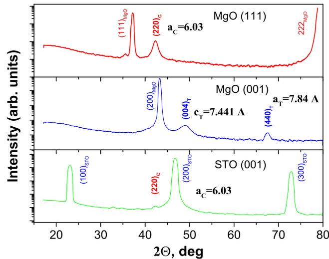
FIG. 1. The X-ray diffraction pattern obtained on 8-nm thick Ni<sub>50</sub>Mn<sub>35</sub>In<sub>15</sub> thin films grown on MgO 111, MgO 001, and STO 001 substrates. The indices and corresponding cubic and tetragonal lattice parameters are presented.
