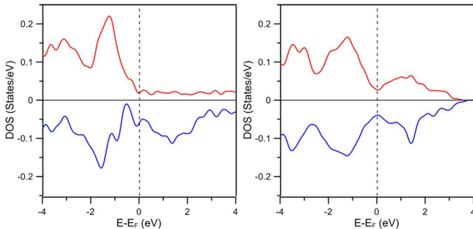
FIG. 4. Local densities of states of the Ni interfacial layer of  $\text{Ni}_2\text{Mn}_{1.5}\text{In}_{0.5}$  films deposited on MgO (001) substrates with two in-plane lattice parameters: 4.21 Å (left), in the FM state, and 4.312 Å (right), in the FiM state.
