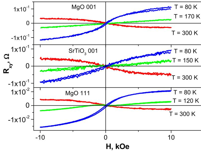
FIG. 3. The Hall resistivity of 8-nm thick  $\text{Ni}_{50}\text{Mn}_{35}\text{In}_{15}$  thin films on different substrates at different temperatures.
