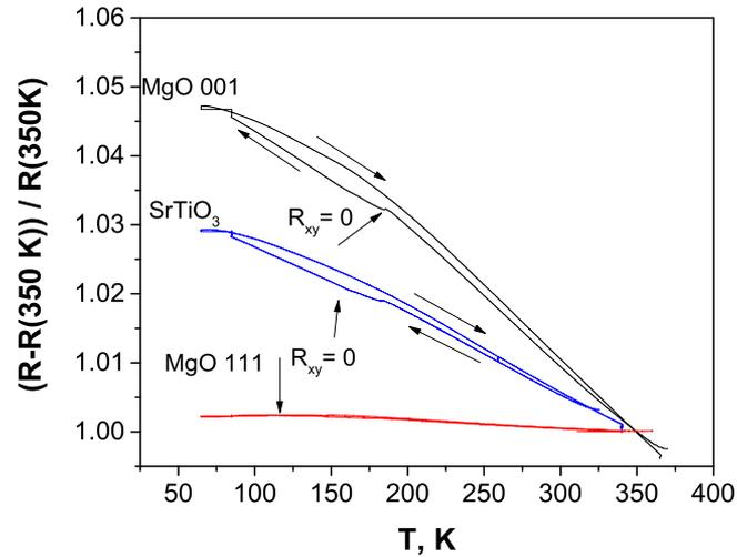
FIG. 2. The temperature dependencies of the resistivity  $\rho(T)$ , normalized to  $\rho(350\text{K})$ . The arrows indicate the temperatures where the AHE ( $R_{xy}$ ) is zeroed-in (see the text).
