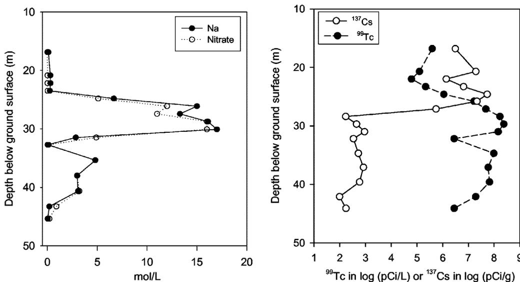
FIG. 2. Porewater concentrations of Na, NO<sub>3</sub>, and <sup>99</sup>Tc [Tc(VII)O<sub>4</sub><sup>-</sup>] in the borehole samples determined by water extraction (46) and laboratory water content measurements. Also shown for reference is the sorbed concentration of <sup>137</sup>Cs determined by high-resolution gamma energy analysis. (Reprinted from reference 46 with permission of the publisher.)
