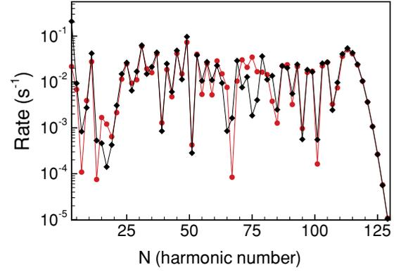
FIG. 2. (Color online) Comparison of exact TS TDER results for HHG rates (circles joined by red lines) with those given by the approximation (29) for  $\chi_N$  (diamonds joined by black lines). The atomic model and laser parameters are the same as in Fig. 1.
