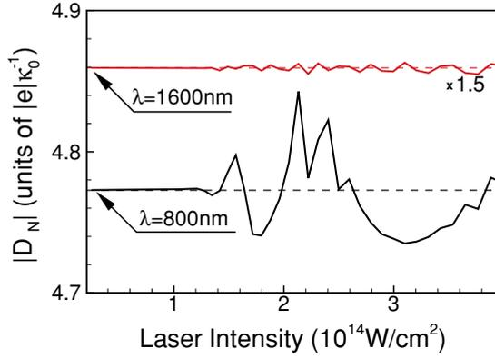
FIG. 3. (Color online) Comparison of the exact result (33) for the absolute value of  $D_N(F, \omega)$  (solid lines) with the approximation (35) (dashed lines), in units of  $|e|\kappa_0^{-1} = 1.065|e|a_B$ . Black lines: results for the 21st harmonic of a laser field with  $\lambda = 800$  nm; red lines: results for the 113th harmonic of a laser field with  $\lambda = 1600$  nm (with these latter results multiplied by a factor 1.5). The parameters of the atomic model are the same as in Fig. 1.
