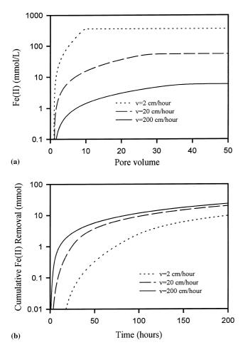
Fig. 6. Fe(II) breakthrough curves and cumulative Fe(II) mass removal from a column subject to iron oxide bioreduction under different flow velocities (see insets). Fig. 6(a) shows breakthrough curves and Fig. 6(b) shows total mass removal from the column  $(K = 7.5 \text{ cm}^3/\text{mmol})$  and other parameters are the same as in Fig. 5).
