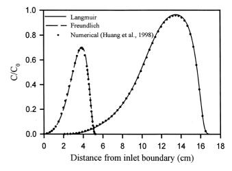
Fig. 4. Concentration distribution (t=190 s) derived from hybrid analytical–numerical solution and Modified Picard Iteration numerical method for cases with nonlinear sorption. (dispersion coefficient,  $D=0.01~{\rm cm}^2/{\rm s}$ ; flow rate,  $v=0.1~{\rm cm/s}$ ; bulk density,  $\rho_b=1.687~{\rm g/cm}^3$ ; porosity,  $\varepsilon=0.37$ ; sorbed concentration,  $S=0.3C^{0.7}$  (Freundlich), =0.3C/(1+100C) mg/kg (Langmuir). (Example after Goode and Konikow [11], Huang et al. [12].)
