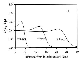
Fig. 3. Concentration changes in a homogeneous porous medium with time-variable parameters. Fig. 3(a) shows a case with L=30 cm D(t)=0.1v(t) cm²/d;  $v(t)=10-8\exp(-t)$  cm/d;  $I(C)=-0.1(1-\exp(-t))C+0.01(1-\exp(-t))$  l/d; R=3;  $f(t)=C_0$ ; Fig. 3(b) shows the same case as in Fig. 4(a) except that  $f(t)=C_a+C_b\exp(-t)$ ,  $C_a=0.4$  and  $C_b=0.6$ .
