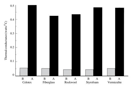
Figure 1. Mean thermal conductance (watts/ $^{0}$ C) of insulated wall panels (n = 20) before (B) and after (A) a 6-month occupation by house mice.
