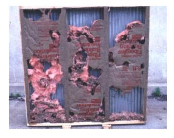
$Figure\ 2.\quad House\ mouse\ damage\ to\ a\ panel\ insulated\ with\ fiberglass\ batt\ after\ 6\ months\ of\ exposure.$
