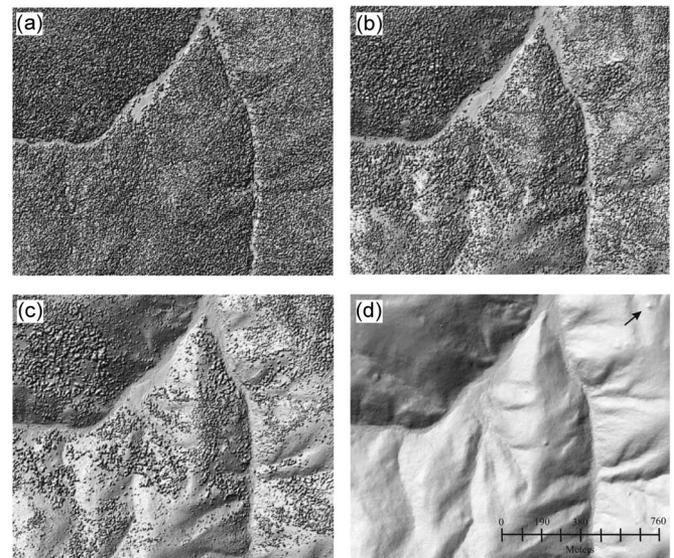
Fig. 4. Shaded relief of interpolated classification results at four stages of MCC operation in each scale domain at the dense forest test site. (a) Preclassified. (b) Convergence in scale domain 1. (c) Convergence in scale domain 2. (d) Convergence in scale domain 3 (final result). The largest potential commission error is indicated by the arrow.
