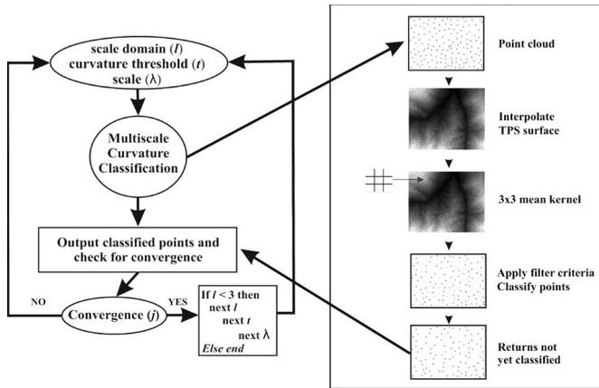
Fig. 2. Flow diagram of the MCC model, where  $l = 1-3$  scale domains, and  $t$  and  $\lambda$  are parameters defining curvature tolerance and scale, respectively.
