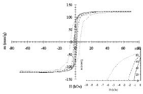
FIG. 4. Hysteresis measurements for two-phase Fe–Pt clusters after different heat treatments showing the development of coercivity. The solid line corresponds to the  $580\,^{\circ}\text{C}/10$  min heat treatment, the dashed line after the additional heat treatment at  $550\,^{\circ}\text{C}$  for 30 min, and the dotted line after the final heat treatment at  $600\,^{\circ}\text{C}$  for 20 min.
