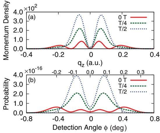
FIG. 2. (Color online) Comparison of (a) the momentum density  $\rho(q_z, t)$  of a coherent superposition of the  $3p$  and  $4p$  states of H (beat period  $T = 6.25$  fs) with (b) the transition probability  $\mathcal{P}$  [cf. Eqs. (3) and (2)] for ( $e, 2e$ ) scattering of a 10 keV, 100 as electron pulse from that state at delay times  $t_d = 0, 1/4$ , and  $1/2 T$ .
