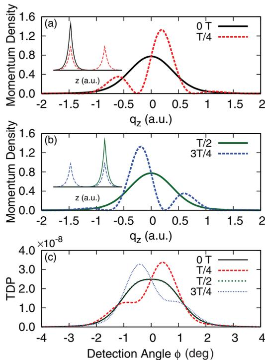
FIG. 4. (Color online) Momentum and charge (inset) densities along the molecular axis of a coherent superposition of  $\text{H}_2^+$   $\sigma_g 1s$  and  $\sigma_u 1s$  states (beat period  $T = 7.1$  fs) for (a)  $t = 0, T/4$  and (b)  $t = T/2, 3T/4$ . (c) The TDP for  $(e,2e)$  scattering of a 10 keV, 100 as electron pulse from that state for four values of the delay time  $t_d$  (cf. Fig. 1 and text for details).
