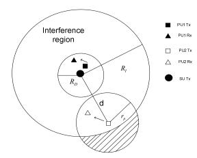
Figure 1. System model of cognitive radio
