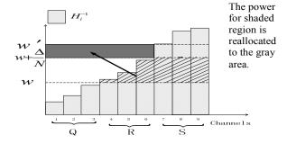
Figure 2. Illustration of power increment water-filling
