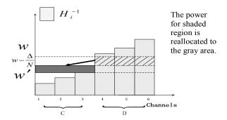
Figure 3. Illustration of Power decrement water-filling
