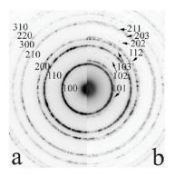
Fig. 1. Electron diffraction patterns of samples  $Zn_{1-x}Mn_xO$  (a) x=0.01 and (b) x=0.03. The patterns are indexed using the wurtzite structure of ZnO. A deteriorated (001) preferred orientation can be noticed with additional rings in (b) in comparison with the pattern in (a).
