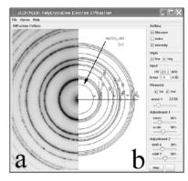
Fig. 2. (a) Electron diffraction pattern of sample  $\rm Zn_{1-x}Mn_xO$ , x=0.05 and (b) a simulated electron diffraction pattern of  $\rm Mn_2O_3$  together with ZnO. The nearest ring in Fig. 2 corresponds to the (211) reflection of  $\rm Mn_2O_3$ .
