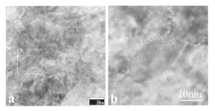
Fig. 4. (a) Plan-view HREM image of sample  $Zn_{1-x}Mn_xO$ , x = 0.05 and (b) enlarged view of a selected area in (a). A secondary phase can be identified in the boundaries of the Mn-doped ZnO phase.
