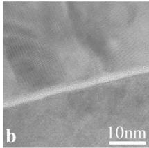
Fig. 5. (a) Cross-sectional HREM image of sample  $Zn_{1-x}Mn_xO$ , x = 0.03 and (b) enlarged view of a selected area in (a). It shows the smooth growth of ZnO grains in a columnar shape on the Si substrate. No precipitate was observed in the interface of Mn-doped ZnO DMS and Si substrate.
