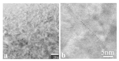
Fig. 3. (a) Plan-view HREM image of sample  $Zn_{1-x}Mn_xO$ , x = 0.01 and (b) enlarged view of a selected area in (a). The hexagonal arrangement of dots or lattice fringes can be viewed in most areas of the grain, and extends to the grain boundaries.
