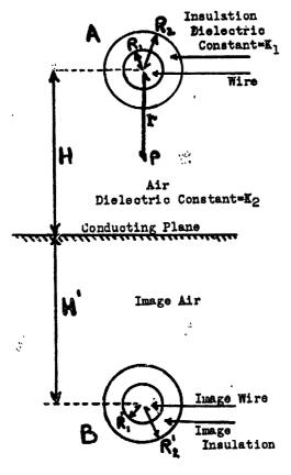
An insulated wire at A is suspended a distance H above and parallel to a plane. The charge on the wire per om. of length is q. In accordance with the method of images, a wire placed baneath the plane at B, directly beneath the wire at A, and a distance H' = H below the plane, with a charge -q per om. of length, will not distort the field.
