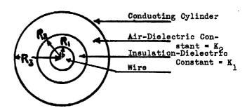
If q is the charge per om. of length, the dielectric flux density at radius r is  $D = \frac{2q}{r}$  lines/cm<sup>2</sup>, and the electric field strength in the medium is  $F = \frac{2q}{Kr}$  dynes, where K has different values in different media. The electric field strength in the air layer,  $F_2$ , is given by  $F_2 = \frac{2q}{K_2r}$ . The electric field strength in the insulating layer,  $F_1$ , is given by  $F_1 = \frac{2q}{K_2r}$ .
