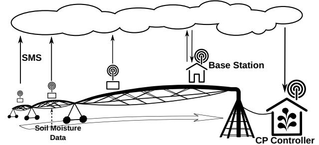
Fig. 1: Overview of the system: aboveground motes attached to the center-pivot collect and relay soil moisture messages from underground motes to the base station.
