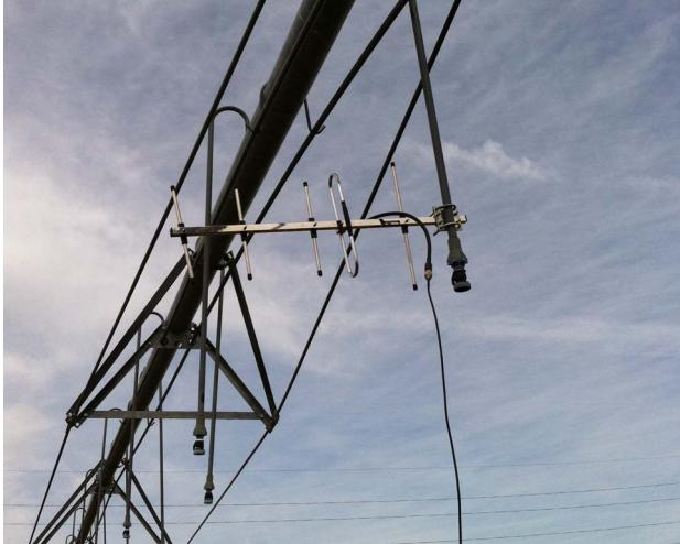
Fig. 4: An aboveground mote attached to the center-pivot.
