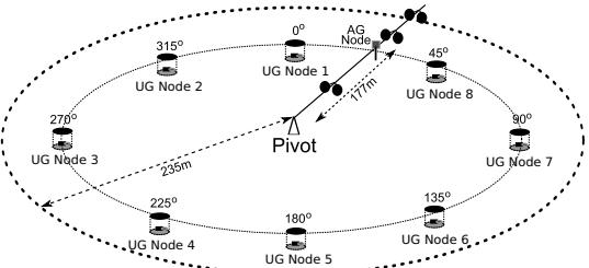
Fig. 3: The setup of the demonstration.
