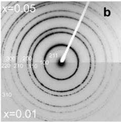
**Figure 4.** Electron diffraction patterns of  $Zn_{1-x}Mn_xO$  thin films. (a) Comparison of x=0.01 (left) and x=0.03 (right). For x=0.01, the diffraction rings are indexed to be (100) to (310) from the centre to the outside; for x=0.03, only the extra diffraction rings that do not appear at the left-hand side are indexed. (b) Comparison of x=0.01 (bottom) and x=0.05 (top). For x=0.05, the innermost diffraction ring is indexed as  $Mn_2O_3$  (211).
