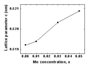
**Figure 2.** Mn concentration dependence of the lattice parameter c of  $\mathrm{Zn}_{1-x}\mathrm{Mn}_x\mathrm{O}$  thin films derived from the (002) spacing.
