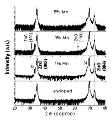
**Figure 1.** X-ray diffraction pattern of  $Zn_{1-x}Mn_xO$  thin films(x = 0, 0.01, 0.03, and 0.05). The intensity axis is plotted on a log scale. The dashed line is plotted to show the shift of the ZnO (004) peak.
