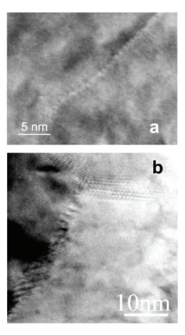
**Figure 3.** High-resolution electron microscopy images of  $Zn_{1-x}Mn_xO$  thin films: (a) x = 0.01; (b) x = 0.05.
