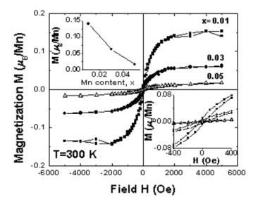
**Figure 5.** Field dependence of magnetization curves of  $Zn_{1-x}Mn_xO$  thin films (x=0.01, 0.03, and 0.05) at 300 K. Top inset: Mn concentration dependence of the saturation magnetic moment of  $Zn_{1-x}Mn_xO$  thin films at 300 K. Bottom inset: enlarged part of the magnetization curves at a low field range.
