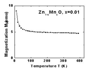
**Figure 6.** Temperature dependence of magnetization curve of a  $Zn_{1-x}Mn_xO$  (x = 0.01) thin film measured at 500 Oe.
