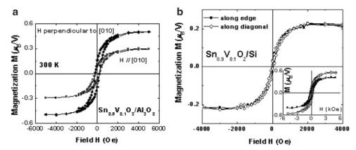
**Figure 4.** Hysteresis loops: (a) at 300 K for the  $\mathrm{Sn_{1-x}V_xO_2}$  (x=0.10) thin film grown on an  $\mathrm{Al_2O_3}$  substrate, with field parallel and perpendicular to the [010] direction, and (b) at 300 K for the  $\mathrm{Sn_{1-x}V_xO_2}$  (x=0.10) thin films grown on Si and  $\mathrm{Al_2O_3}$  (inset) substrates, with field along the edge (solid square) and diagonal (open diamond) of the square samples.
