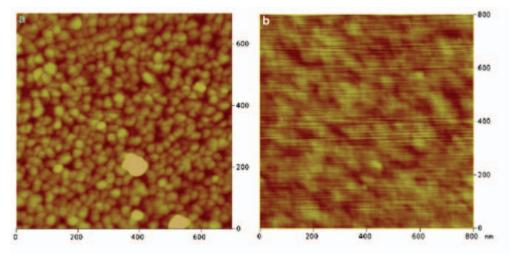
**Figure 2.** AFM images of the  $Sn_{1-x}V_xO_2$  (x=0.10) thin films grown on Si (a) and  $Al_2O_3$  (b) substrates.
