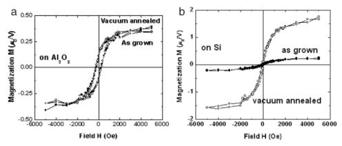
**Figure 5.** Hysteresis loops at 300 K for the  $Sn_{1-x}V_xO_2$  (x = 0.05) thin films grown on (a)  $Al_2O_3$  and (b) Si substrates before (solid circles) and after (open circles) 3 h of vacuum annealing at 500 °C.
