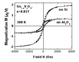
**Figure 3.** Field-dependent magnetization curves at 300 K for the  $\mathrm{Sn_{1-x}V_xO_2}$  (x=0.027) thin films grown on Si and  $\mathrm{Al_2O_3}$  substrates.
