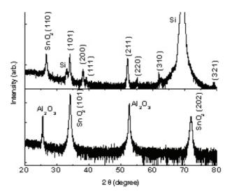
**Figure 1.** XRD patterns of the  $\operatorname{Sn}_{1-x}V_xO_2$  (x=0.10) thin films grown on Si (top panel) and  $\operatorname{Al}_2O_3$  (bottom panel) substrates.
