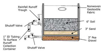
Fig. 3. Cross section schematic of a mesoscale laboratory lysimeter.
