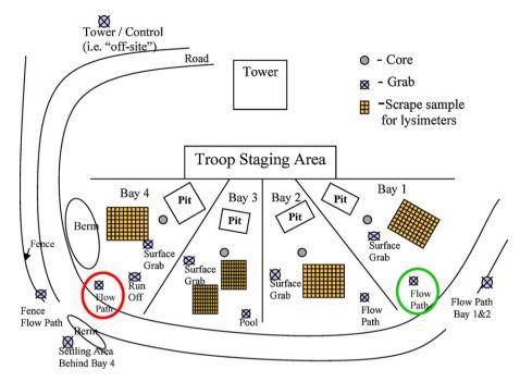
Fig. 1. Schematic of the hand grenade range.
