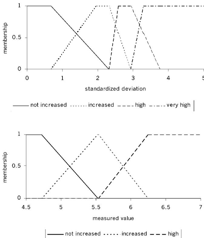
**Figure 4.** Fuzzification of input variables of the right hind quarter as applied in Figure 3 for mastitis alerts: standardized deviation of electrical conductivity (top) and measured value (mS/cm, bottom).
