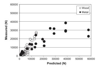
Fig. 8. Comparison of predicted versus measured force for all tests conducted on posts.
