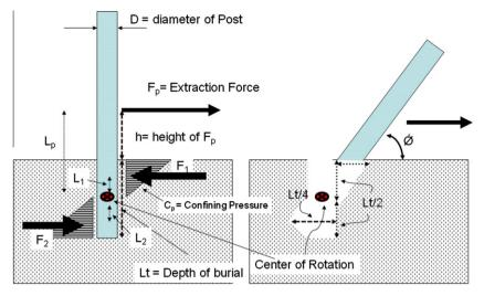
Fig. 2. Force diagram for posts.
