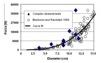
Fig. 1. Diameter of obstacle (tree) versus override force.
