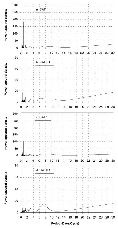
Figure 7. Average power spectral density of the air temperature errors for the HMP45C sensors during the first month.
