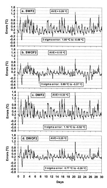
Figure 5. Time series of air temperature errors and statistical values for the HMP45C sensors during the second month.
