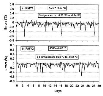
Figure 6. Time series of air temperature errors and statistical values for the RMY temperature system.
