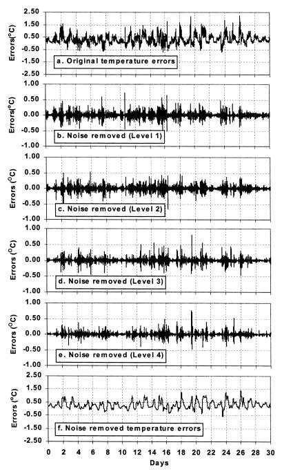
Figure 3. Illustration of noise removal of air temperature errors in measurements. The original signal of air temperature errors illustrated here is from the SWF1.
