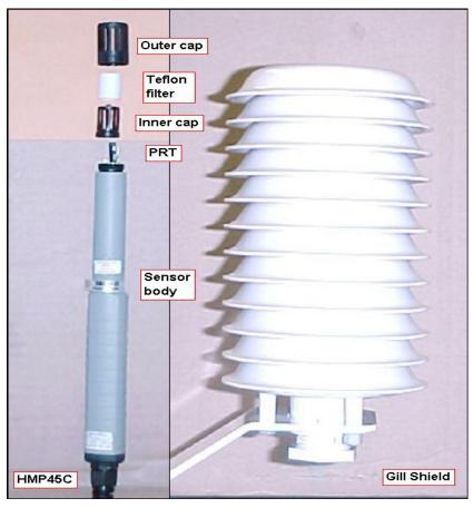
Figure 1. HMP45C sensor and Gill radiation shield.
