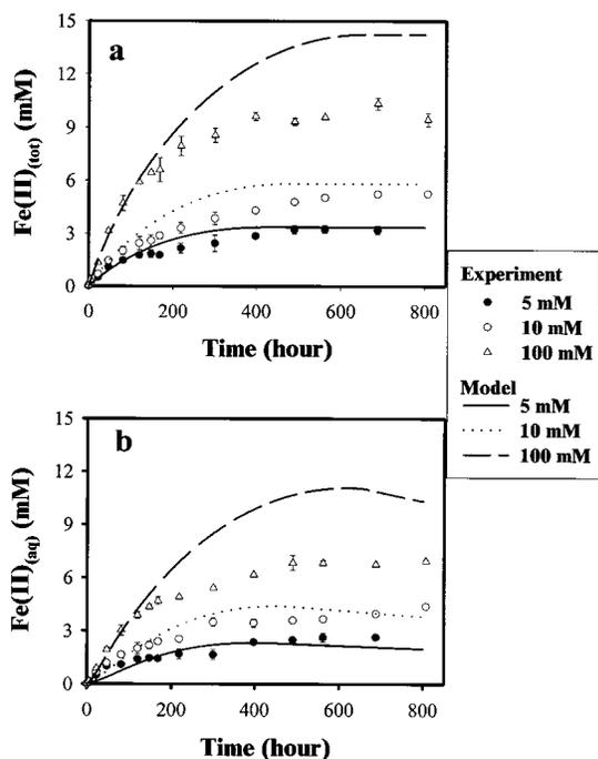
FIGURE 9. Model calculations of goethite reduction by CN32 with variable initial goethite concentrations. The goethite reduction rate was described by eq 3 (text). The siderite precipitation rate and other equilibrium reactions are in Table 1: (a) total Fe(II) and (b) aqueous Fe(II).
