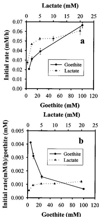
FIGURE 2. Goethite reduction rates as a function of lactate concentration and suspension density (a fixed 30 mM lactate for variable FeOOH cases and a fixed 50 mM FeOOH for variable lactate cases; all cases with 30 mM bicarbonate): (a) overall bioreduction rates and (b) mass normalized reduction rates.
