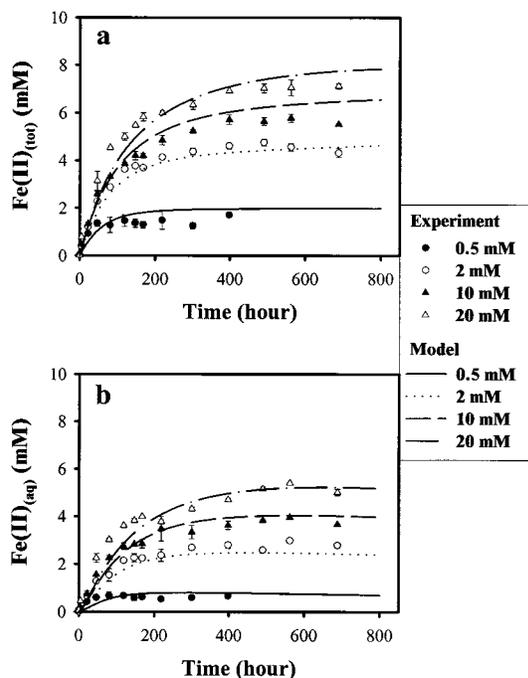
FIGURE 13. Model calculations of goethite reduction by CN32 with variable initial lactate concentrations. Model parameters were the same as in Figure 12.
