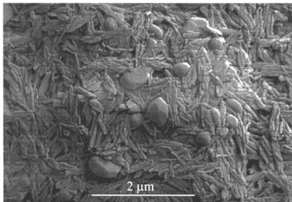
FIGURE 6. Scanning electron micrograph of residual solids after goethite bioreduction. Siderite ( $\text{FeCO}_3$ ) is present as pseudorhomboidal precipitates ranging from 0.25 to 0.5  $\mu\text{m}$  in size.
