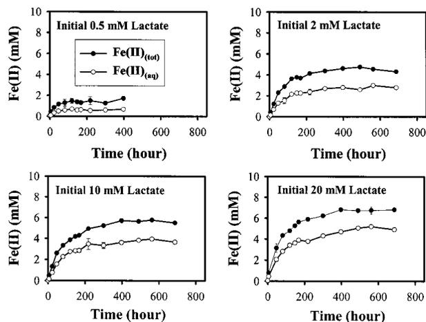
FIGURE 4. Fe(II) production (total and aqueous) in goethite suspensions with variable initial lactate concentrations [goethite = 50 mM and bicarbonate = 30 mM].
