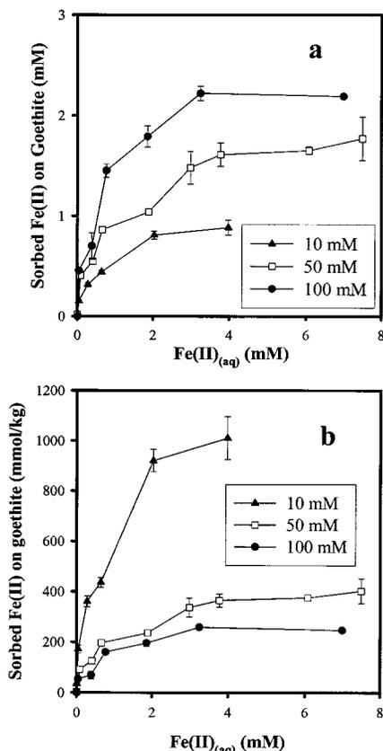
FIGURE 1. The sorption of  $\text{Fe(II)}$  in goethite suspensions of different densities: (a) total concentration isotherm and (b) mass normalized isotherm.
