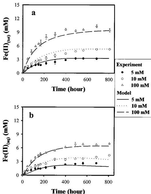
FIGURE 12. Model calculations of goethite reduction by CN32 with variable initial goethite concentrations after the reduction rate was modified with a free energy term eq 6. Other processes are described in Table 1: (a) total Fe(II) and (b) aqueous Fe(II).
