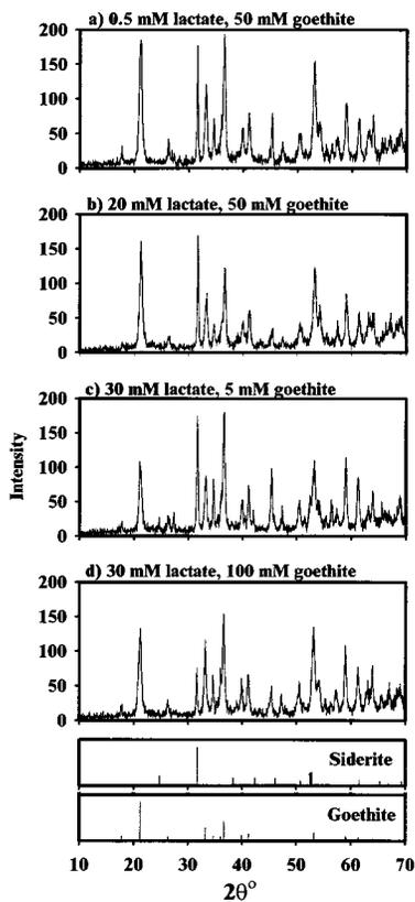
FIGURE 5. X-ray diffractograms of residual solids at the end of goethite bioreduction experiments. Results are shown for variable lactate and variable goethite experiments (goethite and siderite are the crystalline phases present).
