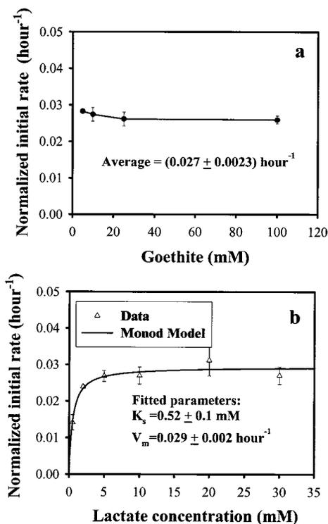
FIGURE 8. (a) The initial rates of bacterial goethite reduction (with 30 mM lactate) normalized by the goethite sorption capacity for Fe(II) (the line is merely connecting data). (b) The normalized initial rates follow Monod type kinetics with respect to lactate concentration. The estimated Monod parameters were 0.029 h<sup>-1</sup> for the maximum reduction rate ( $V_m$ ) and 0.52 mM for the half-saturation constant.
