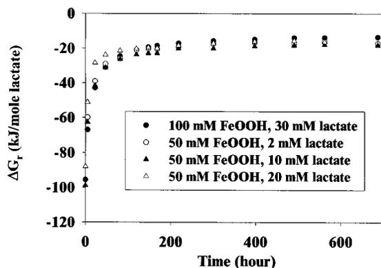
FIGURE 11. Available free energy associated with goethite reduction-lactate oxidation. The reaction free energy was calculated using eq 4 (text), the measured aqueous and total Fe(II) concentrations and reaction stoichiometry (reaction 4).
