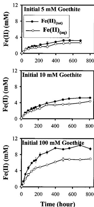
FIGURE 3. Fe(II) production (total and aqueous) in goethite suspensions of different densities [lactate = 30 mM and bicarbonate = 30 mM].
