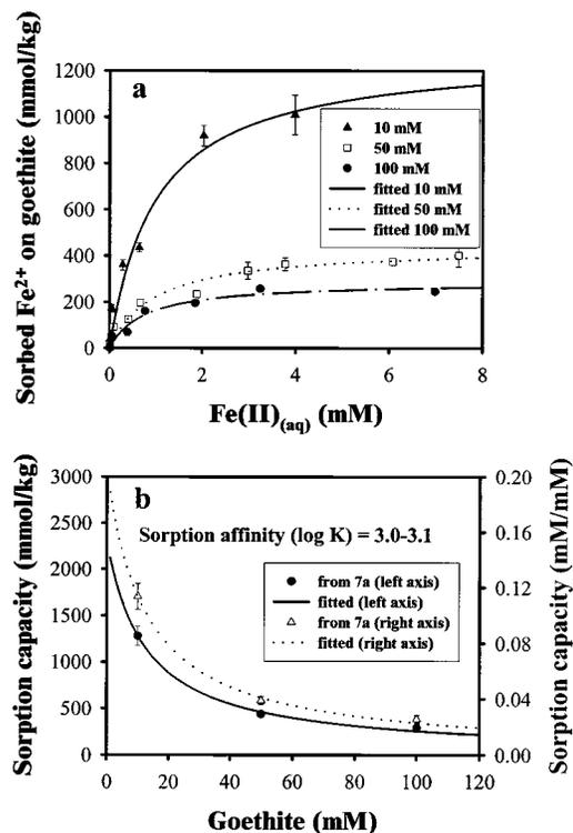
FIGURE 7. (a) Fe(II) sorption data on goethite fitted to the Langmuir isotherm and (b) the fitted Langmuir sorption capacities (from part a) change with goethite concentration and follow a hyperbolic function.
