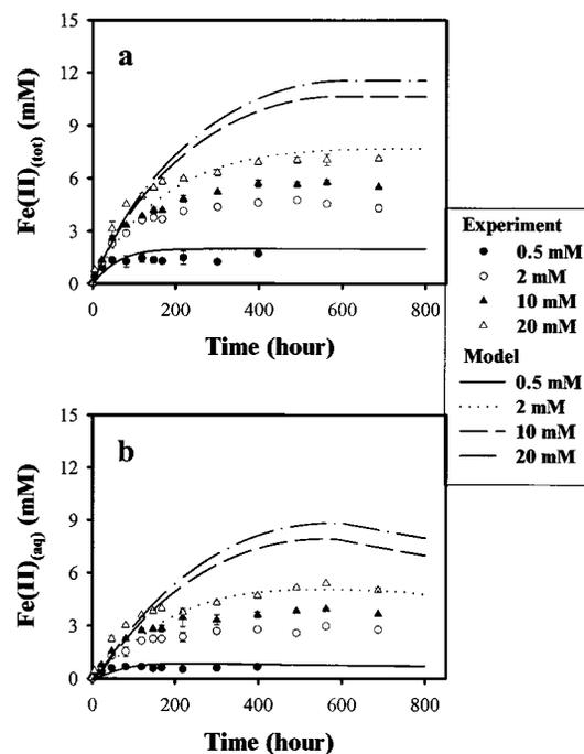
FIGURE 10. Model calculations of goethite reduction by CN32 with variable initial lactate concentrations. The model parameters were the same as in Figure 9.
