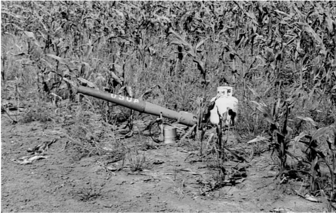
Figure 1. Gas exploder connected to a 9-kg propane tank on edge of a cornfield.
