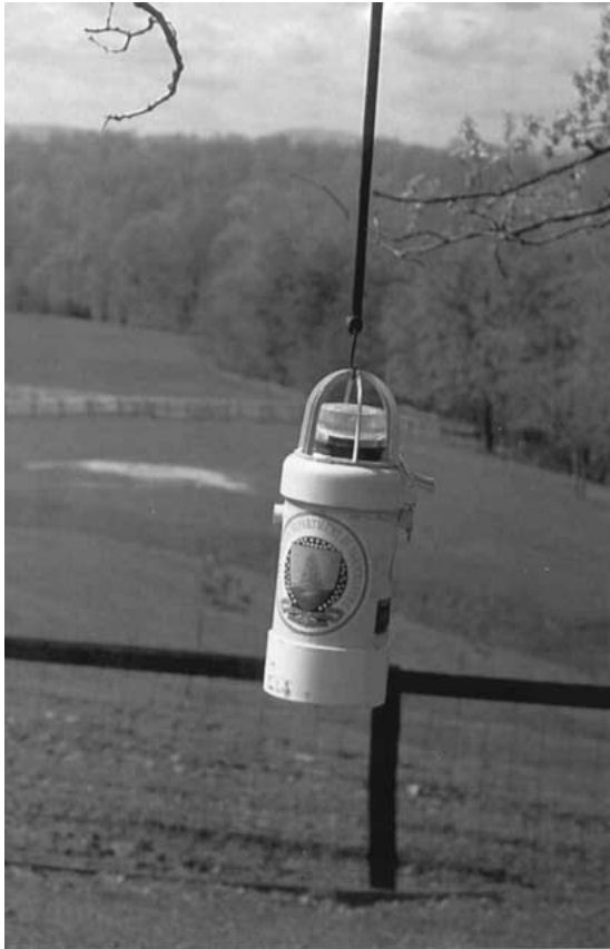
Figure 4. Electronic Guard suspended along sheep pasture. (USDA/APHIS/WS Photo)
