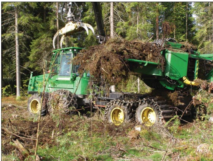
FIGURE 6 | Harvesting of slash materials in Finland using a low ground pressure and tracked Deere bundling system (photo by Daniel G. Neary).
