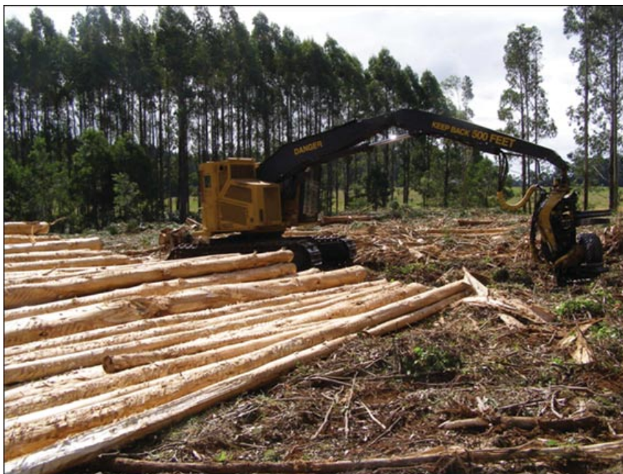
FIGURE 7 | Stacking of a Eucalyptus nitens stems in a SMZ in northern Tasmania, Australia, by a Tigercat tracked harvester (photo by Daniel G. Neary).
