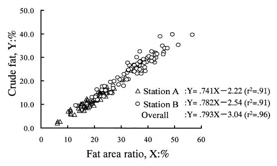
**Figure 1.** Relationship between crude fat content measured with the ether extraction method and fat area ratio calculated with computer image analysis of the ribeye image from two experiment stations.
