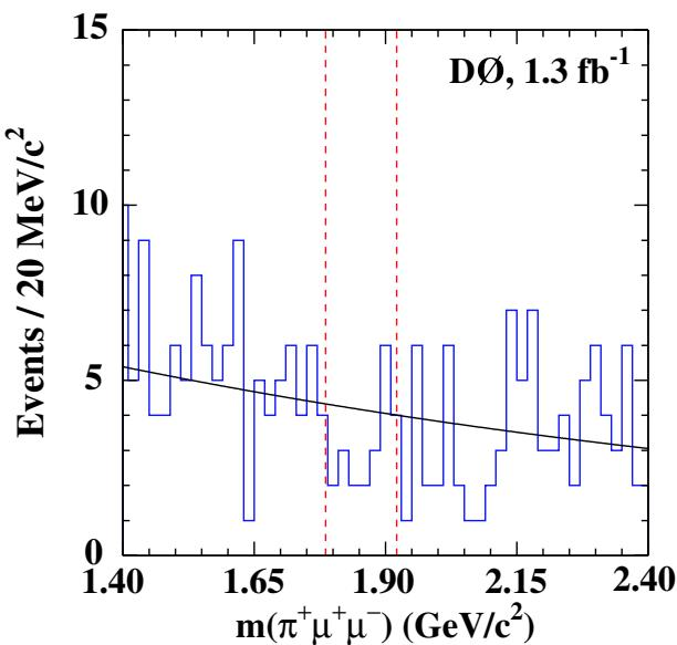
FIG. 3 (color online). Final  $\pi^+\mu^+\mu^-$  invariant mass spectrum. The  $\pm 2\sigma$   $D^+$  signal region, within the dashed lines, contains 19 events. The background level determined from the sidebands is  $25.8 \pm 4.6$  events.
