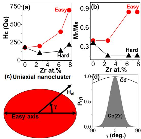
FIG. 3. (a)  $H_c$  and (b)  $M_r/M_s$  at 300 K of Co(Zr) nanoclusters as a function of Zr contents measured along easy (x) and hard (z) axes. (c) Schematic of a uniaxial nanocluster, where  $H_{al}$  is the magnetic field used for alignment and  $\gamma$  is the angle between the easy axis and  $H_{al}$ . (d) The probability distribution  $P(\gamma)$  of easy axes for Co and Co(Zr) nanoclusters having 7.8 at. % of Zr.
