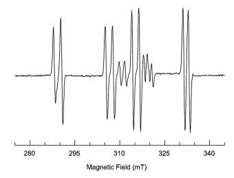
FIG. 3. EPR spectrum of the  $Ag^{2+}$  trapped hole centers. These data were taken at 15 K with the magnetic field along the [101] direction. The four dominant doublets are associated with center A, the isolated  $Ag^{2+}$  ion. The other less intense doublets in this spectrum are assigned to center B.
