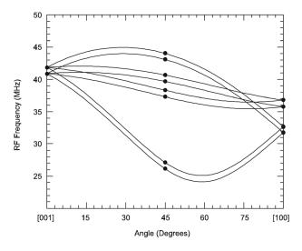
FIG. 6. ENDOR angular dependence in the (010) plane for center A. The solid lines were computer-generated using the g and  $^{109}$ Ag hyperfine parameters in Table I and a microwave frequency of 9.500 GHz. The discrete points are experimental data.
