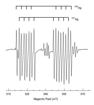
FIG. 7. EPR spectrum from the radiation-induced Ag-related electron trap in a  $\text{Li}_2\text{B}_4\text{O}_7$  crystal. The data were taken at 40 K with the magnetic field along the [001] direction. Stick diagrams indicate hyperfine interactions with  $^{107}\text{Ag}$  and  $^{109}\text{Ag}$  nuclei and with a neighboring I =3/2 nucleus.
