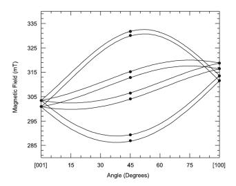
FIG. 5. EPR angular dependence in the (010) plane for center A. The solid lines were computer-generated using the g and  $^{109}$ Ag hyperfine parameters in Table I and a microwave frequency of 9.500 GHz. The discrete points are experimental data.
