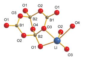
FIG. 1. (Color online) Schematic representation of a portion of the  ${\rm Li}_2 B_4 O_7$  crystal. The five oxygen ions surrounding a lithium site are illustrated along with the basic  $B_4 O_9$  group. This view is along an arbitrary direction.
