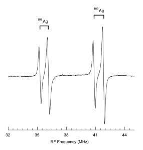
FIG. 4. ENDOR spectrum from center A, the isolated  $Ag^{2^+}$  ion. These data were taken at 15 K while sitting on the low-field EPR line in Fig. 2. The magnetic field was along the [001] direction. Stick diagrams indicate the assignments of lines to the  $^{107}Ag$  and  $^{109}Ag$  nuclei.
