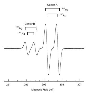
FIG. 2. EPR spectrum showing two similar radiation-induced  $Ag^{2+}$  ions in  $Li_2B_4O_7$  (labeled center A and center B). The data were taken at  $15\,K$  with the magnetic field along the [001] direction. Individual lines due to hyperfine interactions with the  $^{107}Ag$  and  $^{109}Ag$  nuclei are not resolved.
