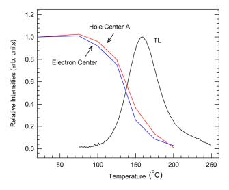
FIG. 8. (Color online) Thermal stabilities of the electron trap and the isolated  $Ag^{2+}$  hole trap (center A) obtained by monitoring their EPR spectra during a sequence of isochronal pulse anneals. Also plotted is the thermoluminescence "glow" curve obtained by monitoring the total light output in the near-ultraviolet region. The effective heating rates are different for the two experiments (see the text for details).
