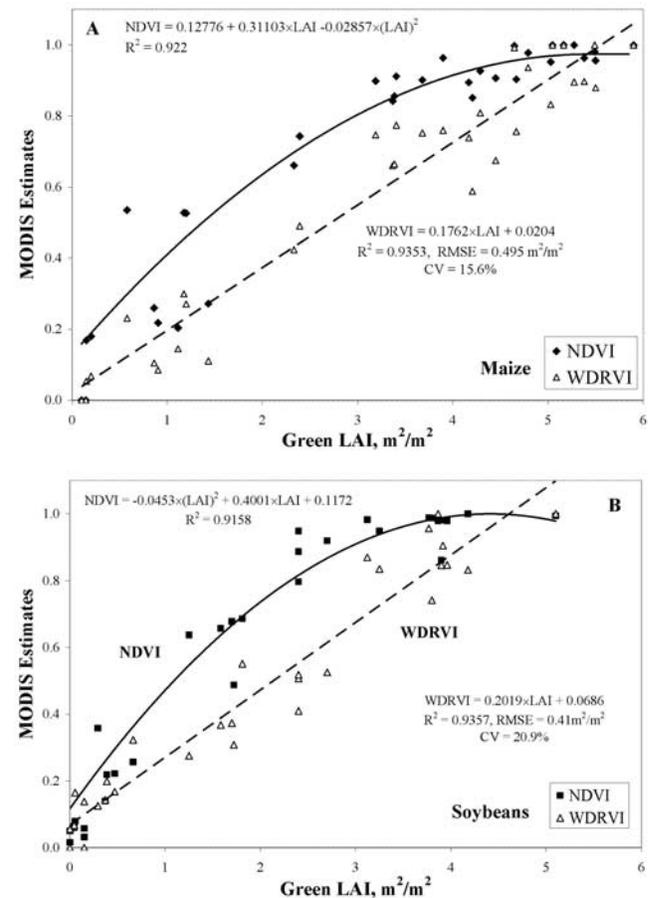
**Figure 3.** Scaled,  $(VI - VI_{\min}) / (VI_{\max} - VI_{\min})$ , NDVI and WDRVI retrieved from MODIS 250-m imagery in (2002 through 2004) plotted versus leaf area index in irrigated and rainfed (a) maize and (b) soybeans. Solid lines are best fit functions for NDVI vs. LAI relations; dashed lines are best fit functions for WDRVI vs. LAI relations.
