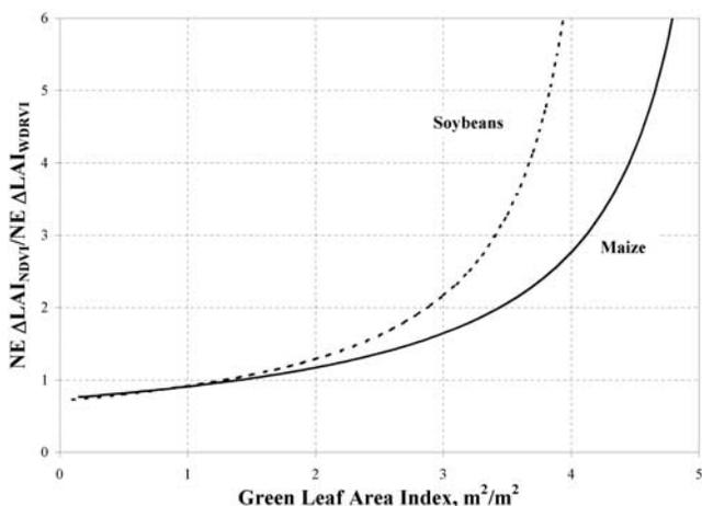
**Figure 4.** Ratio of noise equivalent of leaf area index (LAI) of MODIS-retrieved NDVI ( $NE \Delta LAI_{NDVI}$ ) and WDRVI ( $NE \Delta LAI_{WDRVI}$ ) plotted versus leaf area index in irrigated and rainfed maize and soybean.
