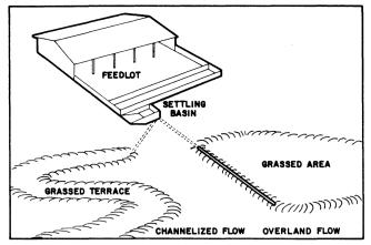
FIG. 1 Vegetative filter configurations for feedlot runoff treatment.
