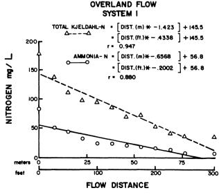
FIG. 2 Nitrogen concentration changes with overland flow (System 1).
