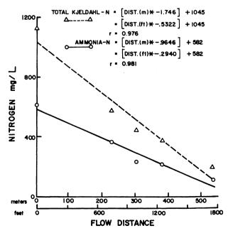
FIG. 3 Nitrogen concentration changes with channelized flow (System 3)
