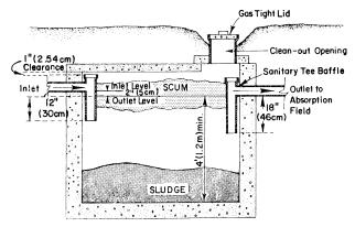
Figure 2. Typical septic tank cross section.
