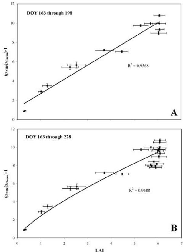
**Figure 4.** The proposed index  $[(\rho_{NIR}/\rho_{green}) - 1]$ , plotted vs. LAI for the data (A) between day of the year (DOY) 163 and 198 before tassels appeared; (B) obtained over the whole growing season. Error bars correspond to two standard errors.
