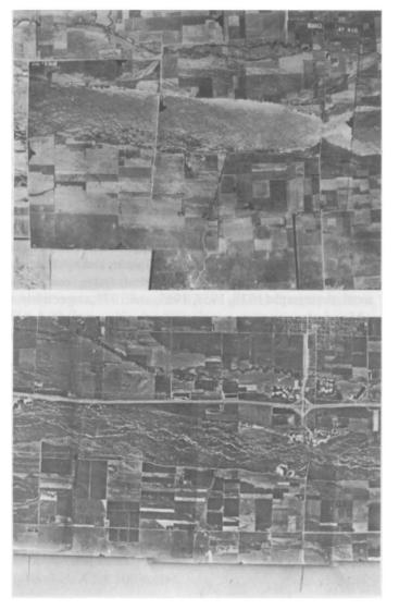
FIGURE 1. Aerial photographs of the Platte River near Kearney, Nebraska, showing change from open channel in 1938 (above) to braided channel interspersed with vegetated islands in 1969 (below). Photos cover about 8 km of river.
