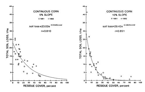
Fig. 6—Soil loss at 51 mm of water applied vs. residue cover.
