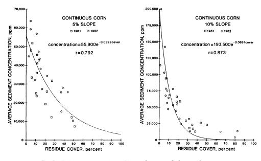
Fig. 7-Sediment concentration at 51 mm of water applied vs. residue cover.
