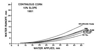
Fig. 4—Cumulative runoff vs. water application for different tillage treatments.
