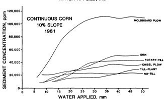
Fig. 5—Sediment concentration in the runoff vs. water application for different tillage treatments.
