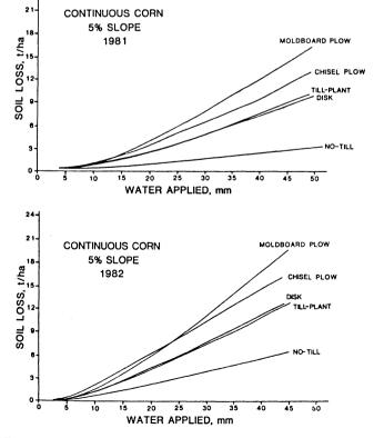
Fig. 2—Cumulative soil loss vs. water application for different tillage treatments evaluated at the Rogers Farm.
