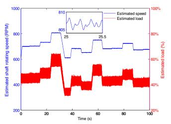
Fig. 10. PMSG input shaft rotating frequency estimated by the PLL method [15] and load estimated by the Hilbert transform [16].
