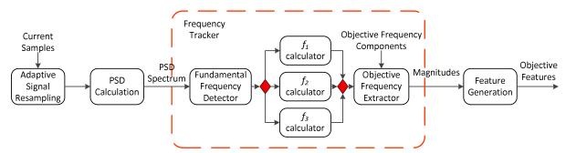
Fig. 3. Schematic diagram of the proposed feature extraction scheme.
