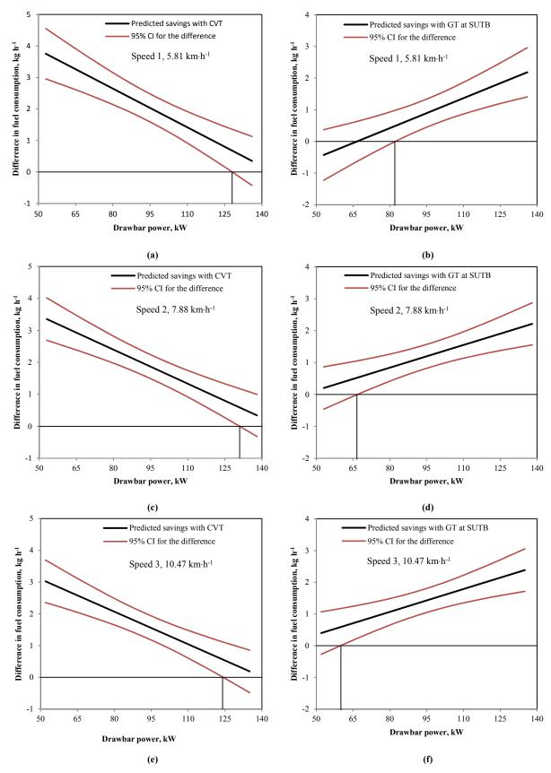
Figure 4. Difference in hourly predicted fuel consumption response to drawbar power between the GT at FT and the CVT (GT at FT – CVT) for (a) speed 1 (5.81 km·h<sup>-1</sup>), (c) speed 2 (7.88 km·h<sup>-1</sup>), and (e) speed 3 (10.47 km·h<sup>-1</sup>) and between the CVT and the GT at SUTB (CVT – GT at SUTB) for (b) speed 1 (5.81 km·h<sup>-1</sup>), (d) speed 2 (7.88 km·h<sup>-1</sup>), and (f) speed 3 (10.47 km·h<sup>-1</sup>).
