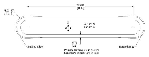
Figure 1. Test track at the Nebraska Tractor Test Laboratory, Lincoln, Nebraska.
