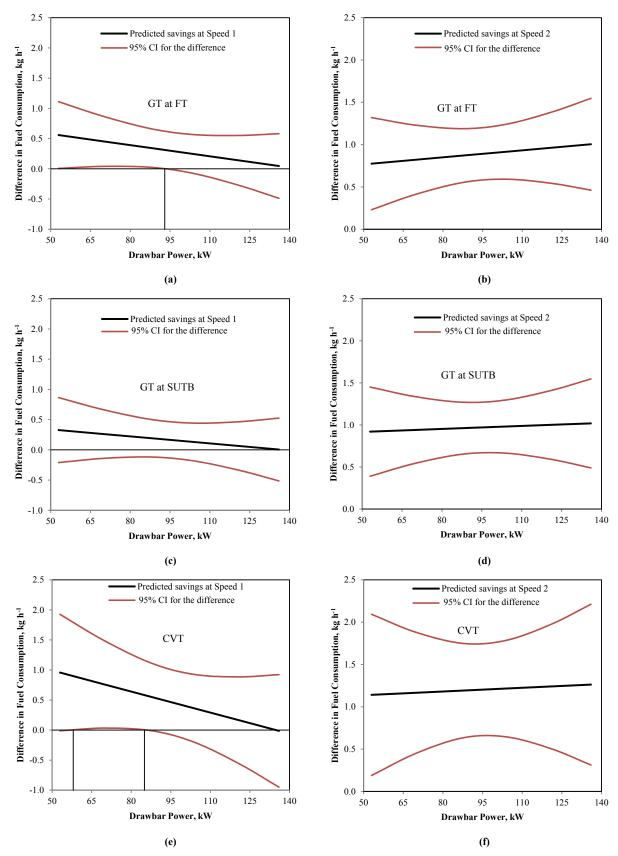
Figure 5. Difference in hourly predicted fuel consumption response to drawbar power between speeds 1 and 2 (speed 2 – speed 1) for (a) GT at FT, (c) GT at SUTB and (e) CVT and between speeds 2 and 3 (speed 3 – speed 2) for (b) GT at FT, (d) GT at SUTB, and (f) CVT.
