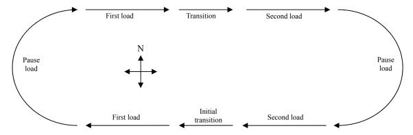
Figure 2. Drawbar load application pattern used (trend continues for the third through sixth loads in randomized sequence of each block) on the test track.
