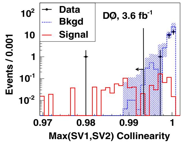
FIG. 3 (color online). The maximum collinearity of the two SVs, for data, background MC, and signal MC with  $M_H = 120$  GeV,  $m_{\text{HV}} = 40$  GeV, and  $L_d = 5$  cm. The hatched region shows the uncertainty on the background MC.
