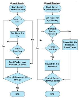
Figure 4. CTC Flowchart of the proposed DPOI algorithm
