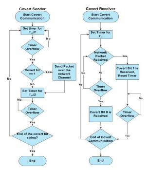
Figure 3. CTC Flowchart of Cabuk et al.'s Algorithm.
