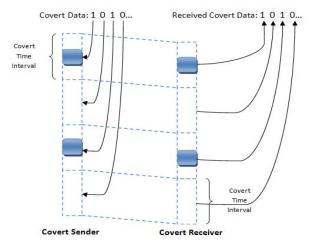
Figure 1. Cabuk et al.'s CTC algorithm (Modified picture from [3])
