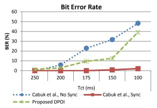
Figure 7. Bit Error Rate for the Covert Timing Algorithms
